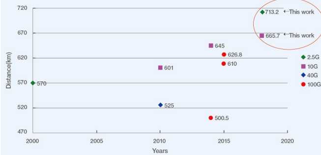
Fig. 3-1 Single-span Unrepeated Laboratory Transmission Test Results for 2.5G and 10G Systems [15]
